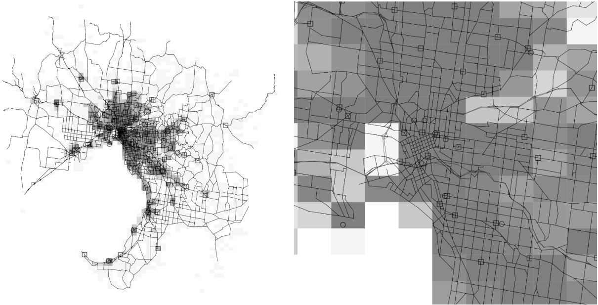
Figure 5 Road network, distribution of demand (darker regions correspond to greater demand), bases (squares), and hospitals (circles) in Melbourne. Left panel: The entire region. Right panel: The city center
